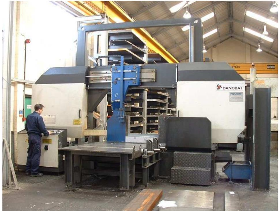
free cutting. This, combined with the 80mm wide blade provides the strength and rigidity for fast accurate cutting up to its 1300mm maximum width capacity. Due to the increased size and weight of material up to 20 tons being handled, heavy duty powered rollerways supplied and manufactured by Prosaw enable the stock material to be easily handled and positioned using a laser.
