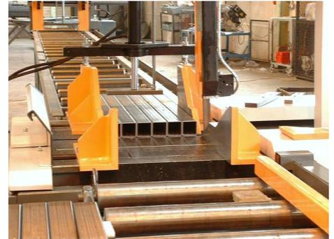
system is totally automatic enabling the operator to carry out other tasks whilst sawing is taking place. An additional benefit is that the crane and forklift are freed up to carry out other tasks.
