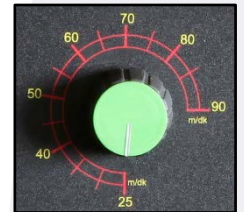
Inverter Speed Control
