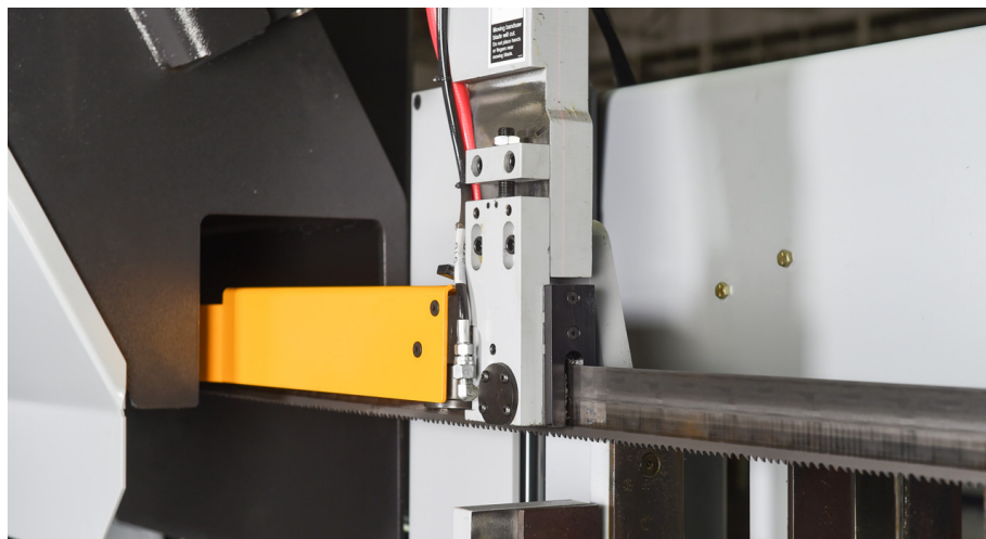
Guide arm is connected to moveable vice for proper spacing
