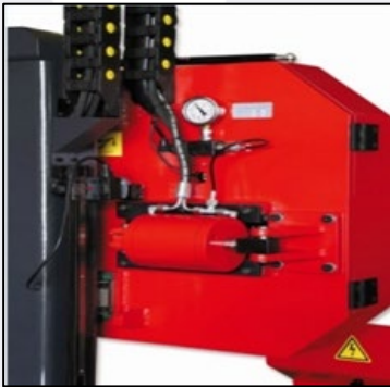
Hydraulic Blade Tensioning
