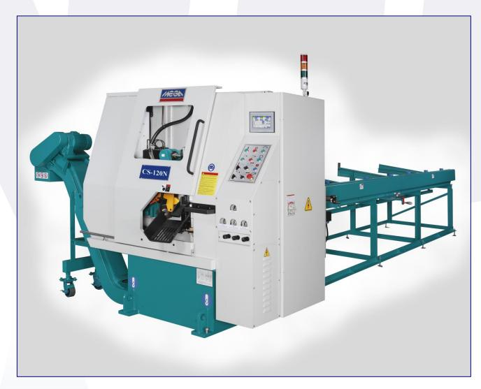
The **Mega CS-120N** is a heavy duty precision cutting machine with excellent repeatability by means of an NC controlled servo motor.
