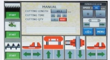
Touch screen control panel
