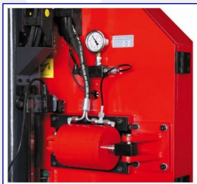
Hydraulic Blade Tensioning
