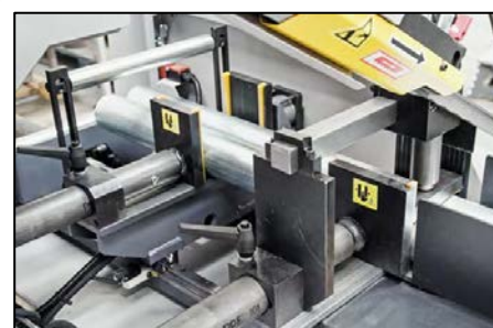
Automatic vice with 500mm stroke
