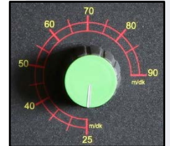
Inverter Speed Control
