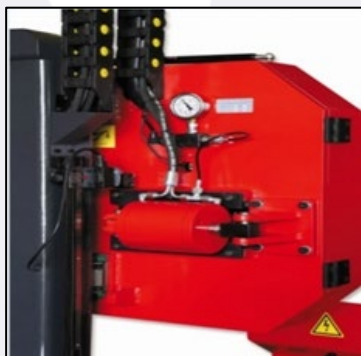
Hydraulic Blade Tensioning
