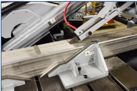
Powered moveable guide arm
