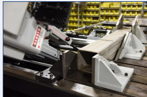
Four full stroking hydraulic vices
