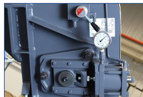
Hydraulic Blade Tension
