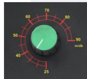
Inverter speed control
